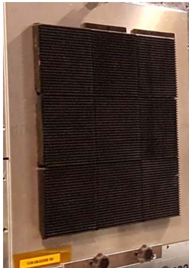
Figure 2-1. Detail of the TK RAM absorber
