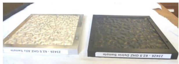
Figure 7 Rough Reference samples 62.5 GHz. Left aluminium, right Dielectric
