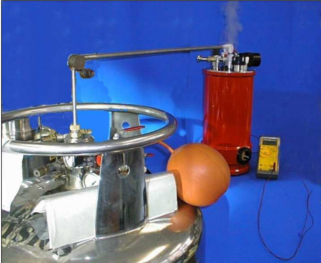
Photo 4.1. Liquid helium transfer
