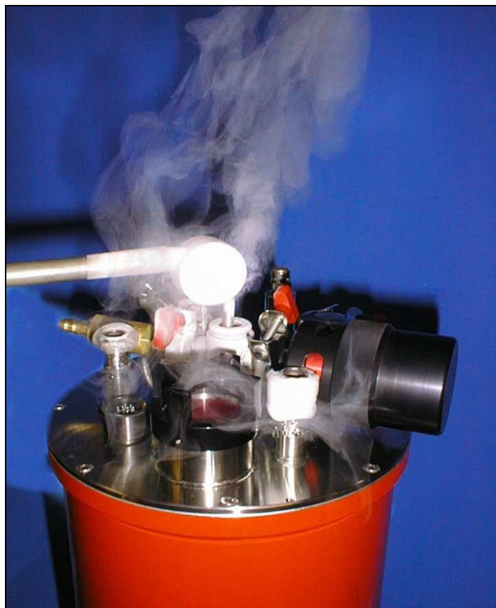
Photo 4.2. Helium gas exhaust during fill
