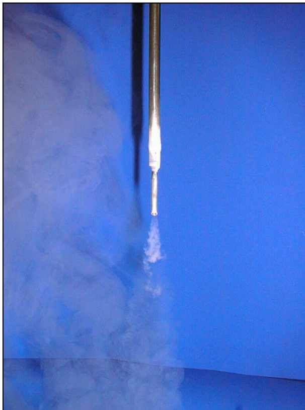
Photo 4.4. Liquid helium emerging from a cold tube
