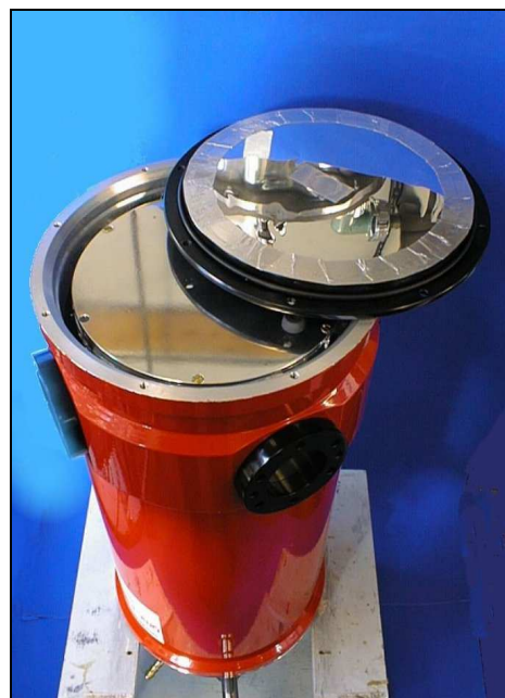
Photo 1.4. Liquid nitrogen base-plate in position
