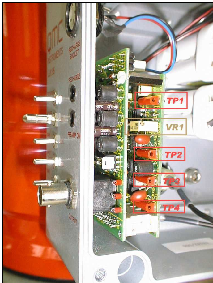
Photo 5.3. View of the switchboard and amplifier circuit board identifying the voltage test points and multi turn potentiometer
