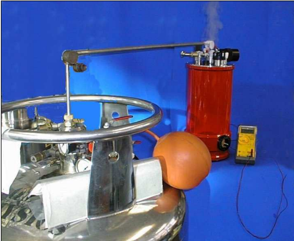
Photo 4.1. Liquid helium transfer
