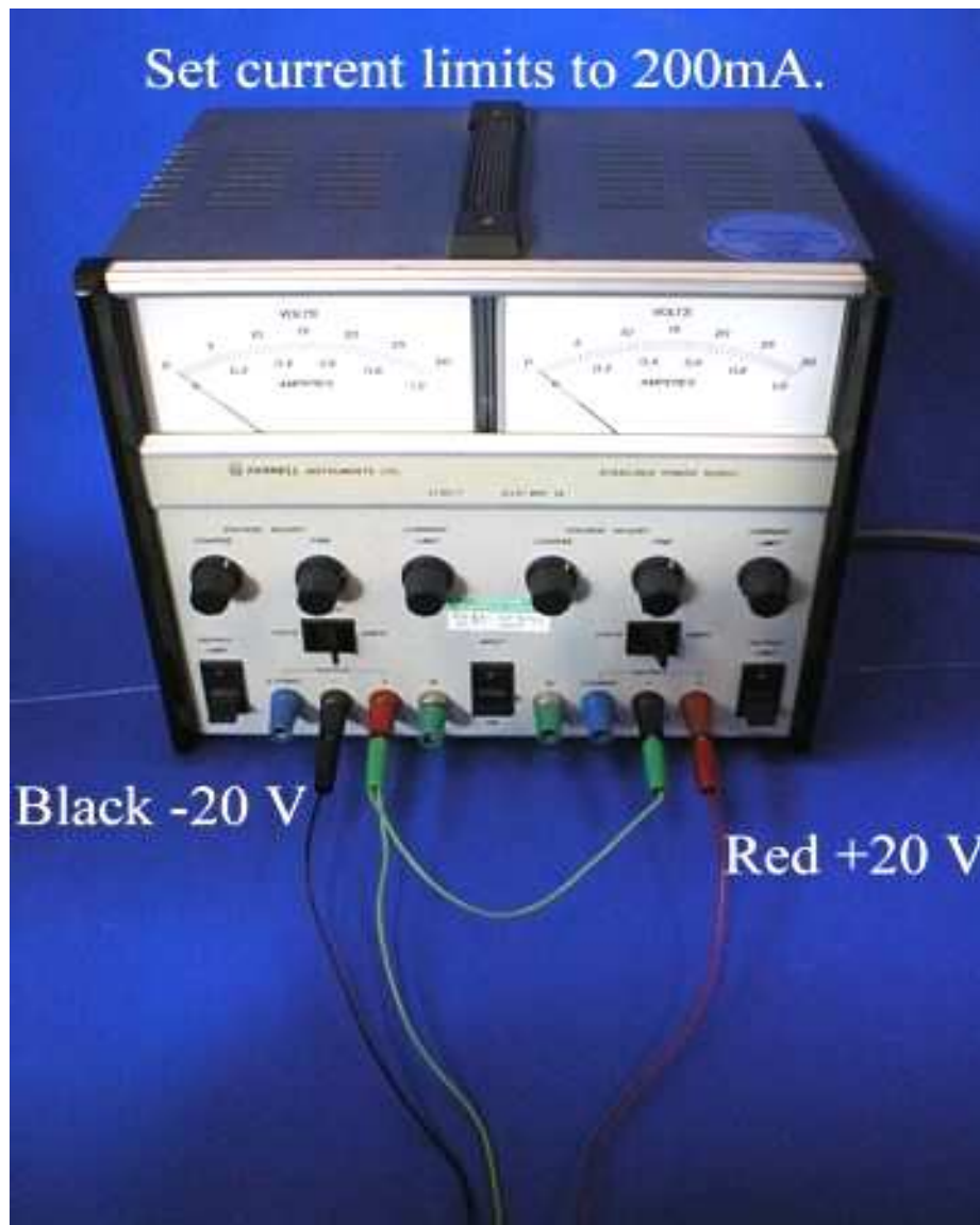
Photo 5.2. Power supply connections
