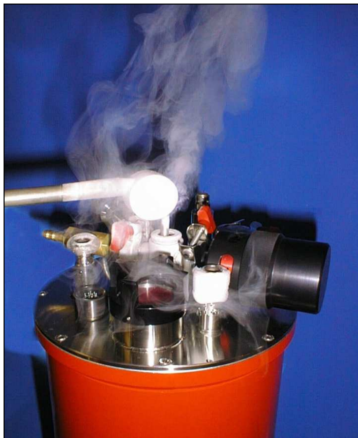
Photo 4.2. Helium gas exhaust during fill
